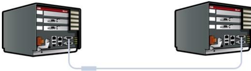
Figure 17 Serial 1 to serial 1 redundant link connections with ferrite core
