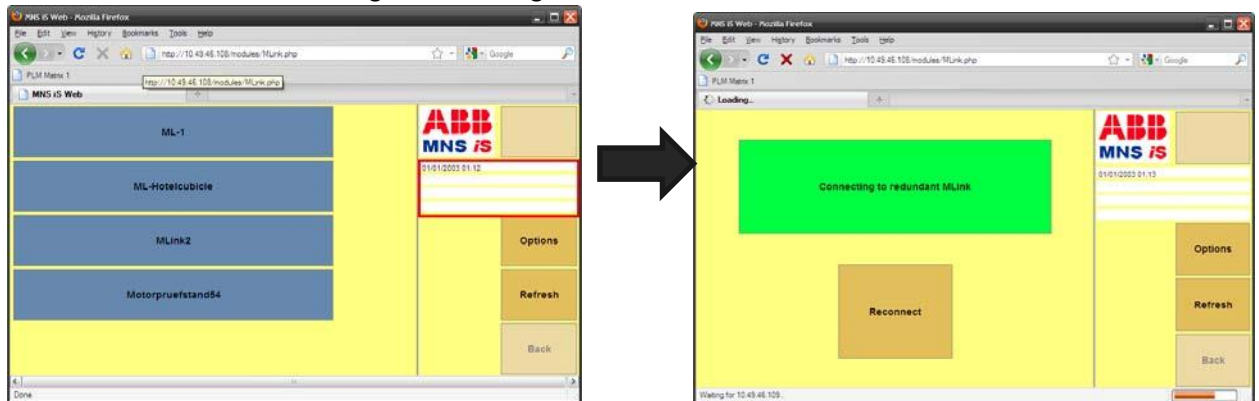
Figure 20 MView Redirecting to Redundant Digital Gateway
