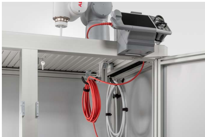
On the inside of the workstation are many options for equipment fixtures and holders
